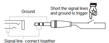
The measurement starts after connecting a signal cable to ground and stops upon disconnection. Note that when the **Trigger** function is active, the **<START/STOP>** key is unavailable.
