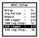
The MEAS.Setup menu is the most important for the measurement. Here you can set the following parameters: Delay, Integration Period, Repeat, SW Log.Step, SWN Log.Step, CSD Logger and CSD Log.Step. You can choose the options by pressing the navigation keys <▲> and <▼>.
