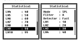
A fixed data source set for statistical purposes is the SPL. The user cannot change this setting. However, in this menu the user can define the SPL detector and filter as well as the statistical value.
