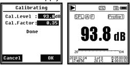
(6) To start the measurement, open the **home screen** again and press <**START/STOP>**. If the calibrator works properly, for the example given in this manual the current measurement result is 93.8 dB.
