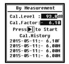
To open this menu, select **By Measurement** and press **<EN-TER>**. Further details concerning the calibrator used and the appropriate adaptation value are provided in <u>Appendix 2</u>, <u>Adaptation of Control Calibration Frequency</u>.
