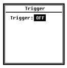
The **Trigger** menu allows you to activate or deactivate the trigger function. **Trigger** is the analogue input which, using remote control commands, enables starting or stopping a measurement performed with the sound level meter. The trigger input is located in at the bottom of the meter (3.5 mm headphone port).
