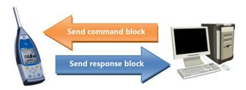
A typical command block or response block consists of a start-of-text character, identifier (ID), attribute character, command or data, end-of-text character, block check character, line feed character and carriage return character, as per the diagram below:
