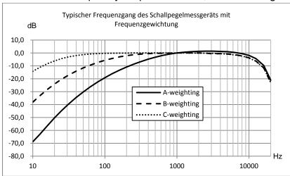
The table below presents the impact of the upper limit of measuring range with A, B and C weightings and the typical frequency response shown in the figure:
