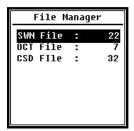
The **File Manager** allows you to manage the saved SWN, OCT and CSD files. The figures given in each line on the right indicates the number of files of each type. With the navigation keys  $< \blacktriangle >$  and  $< \blacktriangledown >$ , you can choose the option and open the next menu level by pressing <ENTER>.
