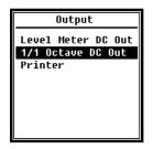
The **Output** menu allows you to choose the measurement data sent to the **DC OUT**. For the **level meter** and **1/1-octave** modes, the options specify the DC output of the level meter and the 1/1-octave DC output.
