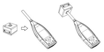
(2) Switch on the calibrator and set a fixed sound level (e.g. 94 dB).
