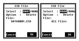
In the **CSD File** menu, you can delete, display or print the content of the CSD file. By pressing the navigation keys <▲> and <▼>, you can move the cursor between **Select** and **Option**. The deletion procedure is the same as for the **SWN File**.
