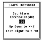
If the measurement results for Profiles 1–3 exceed the **Alarm Threshold**, the red LED above the **<POWER>** key will light up. The alarm threshold can be set within a range from 20 dB to 200 dB. With the navigation keys <▲> and <▼>, you can increase or reduce the alarm threshold by 1 dB. With the navigation keys <◄> and <▶>, you can increase or reduce the setting by 10 dB.
