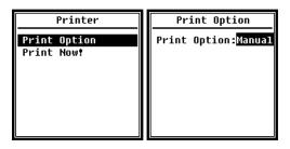
The **Print** option allows to set the automatic or manual printing mode. If you choose **Auto**, the measurement results will be printed automatically once the measurement is stopped.
