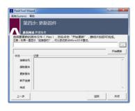
**Step 4:** Press the key located in the upper right corner to choose the firmware, and then press **Update** to start the program. The whole procedure takes 3 to 4 minutes.
