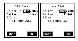
To display or print the content of the CSD file, select **Option** in the **CSD File** menu and press the navigation keys <◀> and <▶>.
