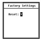
The **Factory Settings** menu allows you to reset all the parameters previously changed by the user and restore the factory settings. The parameters will be initiated with the standard values. By pressing the navigation keys <◀> and <▶>, you can choose Y (Yes) or N (No). The parameters will be initiated after selecting Y (Yes) and pressing **<ENTER>**. By selecting N (No) or pressing
