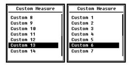
The **Custom Measure** menu offers 14 options where you can define the parameters for 1–14 custom measurements. With the navigation keys <**△**> and <**▼**>, you can choose the option and open the next menu level by pressing **<EN-TER**>.
