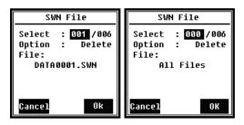
In the **SWN File** menu, you can delete the SWN files using the navigation keys <▲> and <▼>. Select the number of the file to be deleted. You will see the file number at the bottom edge of the screen. If you enter 0000 as the file number, you will delete all the available SWN files.
