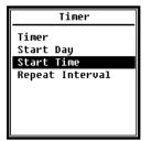
In the timer menu, the **Timer** option allows you to set the **Start Day**, **Start Time** and **Repeat Interval**. Press the navigation keys <▲> and <▼> to choose the option.
