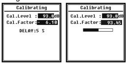
(5) When it is completed, the calibration factor in the sound level meter will be updated. Press **<ENTER>** to apply the results.
