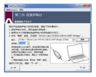
**Step 3:** Connect the sound level meter to the computer as per the user requirements. Note that the sound level meter requires an external power supply. If the driver works properly, it will automatically select the CP210x **port**. The standard **baud rate** is 115,200 bps, but it depends on the computer. A higher **baud rate** allows for a faster updating procedure.
