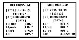
With the navigation keys <▲>, <▼>, <◄> and <►>, you can view the file content in the View mode. The **Print** mode is almost identical to the **View** mode. Press **<Enter>** to print the content of the currently displayed CSD file.
