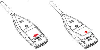
Turn the lock right to enable cover removal. Remove the cover from the battery container.
