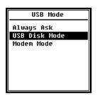
In the **USB Mode** menu, you can set the operating mode of the sound level meter connected to a computer using a USB cable. The following options are available: **Always Ask**, **USB Disk Mode** and **Modem Mode**.
