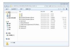
Unpack and install the driver according to the following procedure. Select the X86 version for a 32-bit operating system or the X64 version for a 64-bit operating system.
