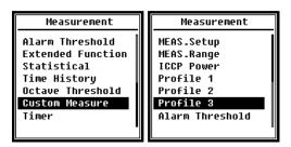
The **Measurement** menu includes 13 options. Using the navigation keys  $< \blacktriangle >$  and  $< \blacktriangledown >$ , you can choose the options and open the next menu by pressing <ENTER>.
