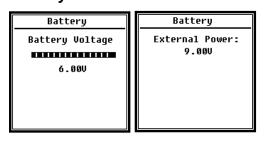
The **Battery** menu shows the battery status and voltage. The final voltage of a single LR6/AA/AM3 battery cell is approx. 0.9 V, so the sound level meter is automatically switched off when the total voltage at 4 cells of the alkaline battery drops below 3.6 V.
