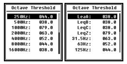
In the **Octave Threshold** menu, you can set the alarm threshold within a range from 31.5 Hz to 16 kHz as well as parameters LAeq, LBeq, LCeq and LZeq. If the measurement result exceeds the threshold, a red LED will light up. By pressing the navigation keys <◄> and <▶>, you can
