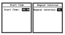
Set the **Start Time** to **00:00**. This is the time when the measurement will be initially activated. In order for the measurement to be reactivated every hour, set **Repeat Interval** to **1** h.
