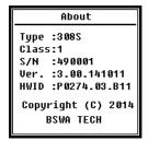
In the "About" menu, you can see the following information: type, class, serial number, version and HWID (hardware ID) of the sound level meter.
