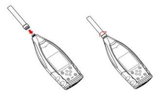
Connect the microphone to the TNC connector. Then turn it on the thread, firmly connecting both elements.
