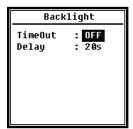
The backlight of the sound level meter is automatically switched off to reduce power consumption and to save the batteries.
