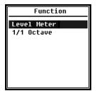
Select **Function** and press **<ENTER>** to open this menu. You can choose 2 types of measurement. **Level measurement** and **1/1-octave measurement**. Press the navigation keys **<**▲**>** and **<**▼**>** to choose the measurement mode. Press **<ENTER>** to save the setting and return to the previous menu. Press **<ESC>** to return to the previous menu.
