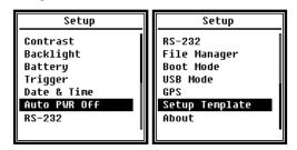
The **Setup** menu allows you to set the main function and conditional display. With the navigation keys <▲> and <▼>, you can choose the option and open the next menu level by pressing <**ENTER>**.
