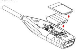
Replace the batteries and then close and lock the battery container cover.
