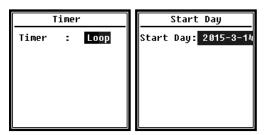
In order to always restart the measurement, set the **Timer** to **Loop**.
